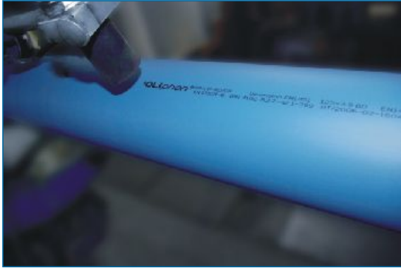
Photo 22. POLlphon pipe - in the course of marking
