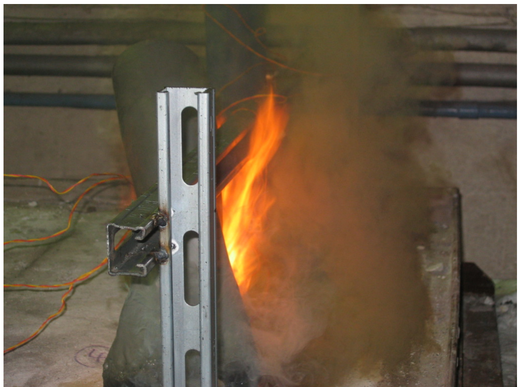
Integrity failure of pipe H after a duration of 231 minutes
