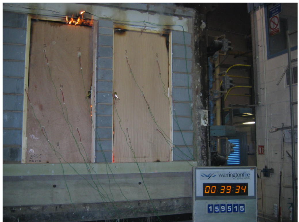
The unexposed face of the doorsets after 39 minutes of testing
